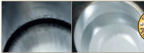
The forcing cone of the competition is pitted and damaged beyond repair after 500 rounds of steel shot.
