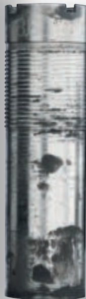
Competitor's tube after extensive shooting
