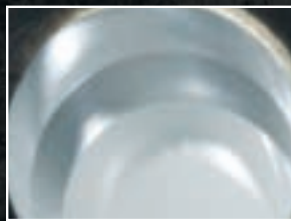
After 500 rounds of steel shot, the higher-quality Browning barrel shows no wear.
