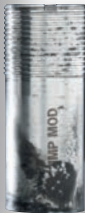
Competitor's tube after extensive shooting
